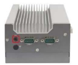
This connector supports Line-in and Line-out. Line-out supports a 2W speaker. Please see diagram below.
